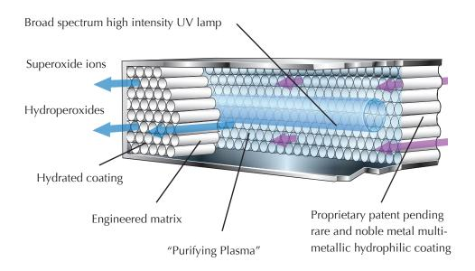
By engineering the proper light wavelengths into the ActivePure cell, activTek Environmental has developed a highly effective system designed to utilize germicidal UV light. Falling between visible UV light and invisible X-Rays in the light spectrum, UV makes use of the same oxidation and
